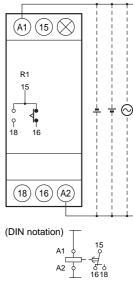
Note 1: The above figure shows the terminal arrangement for a 24 to 48-VAC/DC model. Models with 100 to 120-VAC or 200 to 240-VAC power input do not have a DC input.
