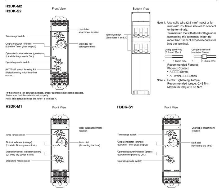
\*If the switch is left between settings, proper operation may not be possible. Make sure that the switch is set properly. Note: The default settings are for 0.1 s in mode A.
