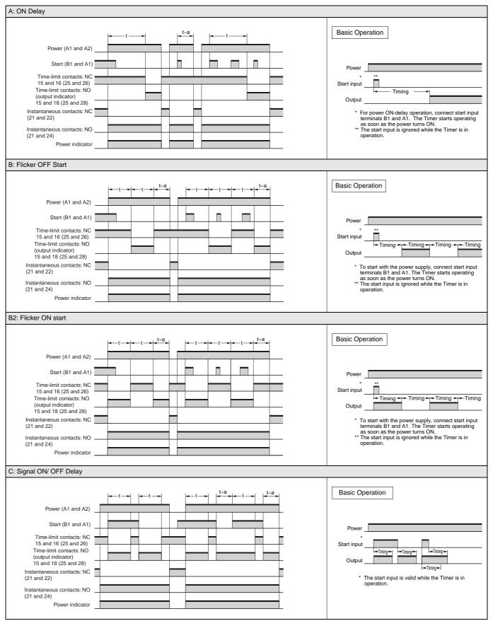
Note 1.The reset time is 0.1 s min. Make sure the signal input time is 0.05 s or longer. Note 2."t" is the set time. "t-a" is a time that is less that the set time.
