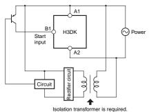
• The H3DK-H has a large inrush current. Provide sufficient power supply capacity.
