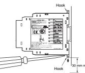
It will be easier to mount and dismount the Timer if a distance of 30 mm or more is provided between the bottom of the Timer and other equipment.
