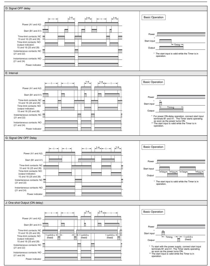
Note 1.The reset time is 0.1 s min. Make sure the signal input time is 0.05 s or longer.
